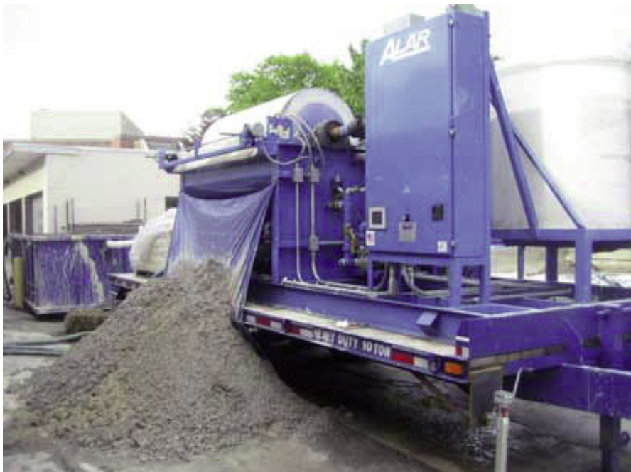
This trailer-mounted Auto-Vac® produces dry, manageable landfill-ready solids, which is easily collected for transport off site.
