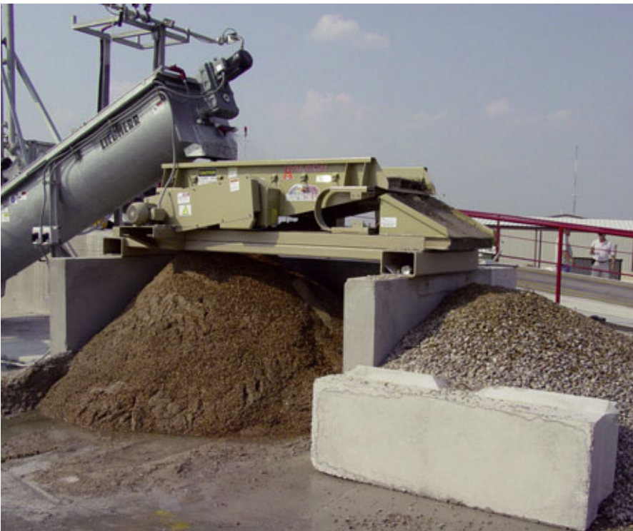
The Liebherr LRS Recycler separates out the rock chips and other aggregate materials and produces a clean, readily transported or recycled material. The concrete chips (circled above) are easily collected and used as fill or recycled.
