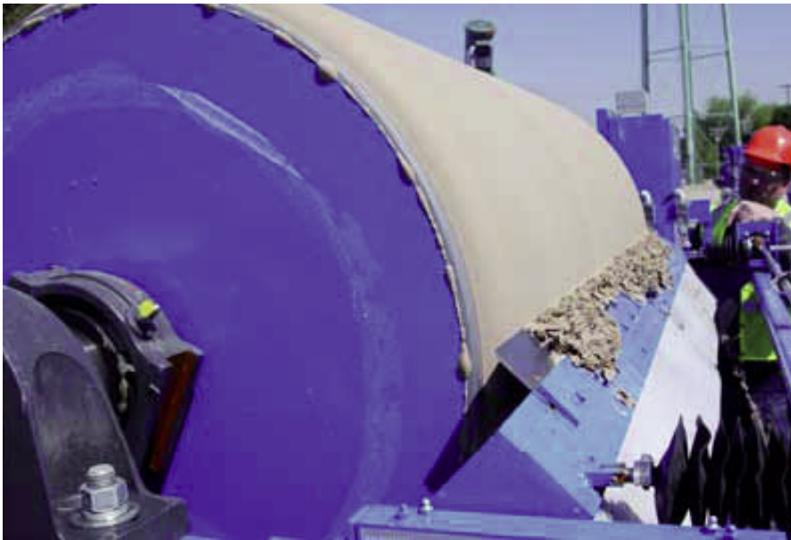
The Auto-Vac® filter separates the cement fine solids from the water. As water is vacuumed through a filter aid media pre-coat, solids accumulate on the drum's surface. A variable speed knife advances, removing the solids from the surface with lathe-like precision.
